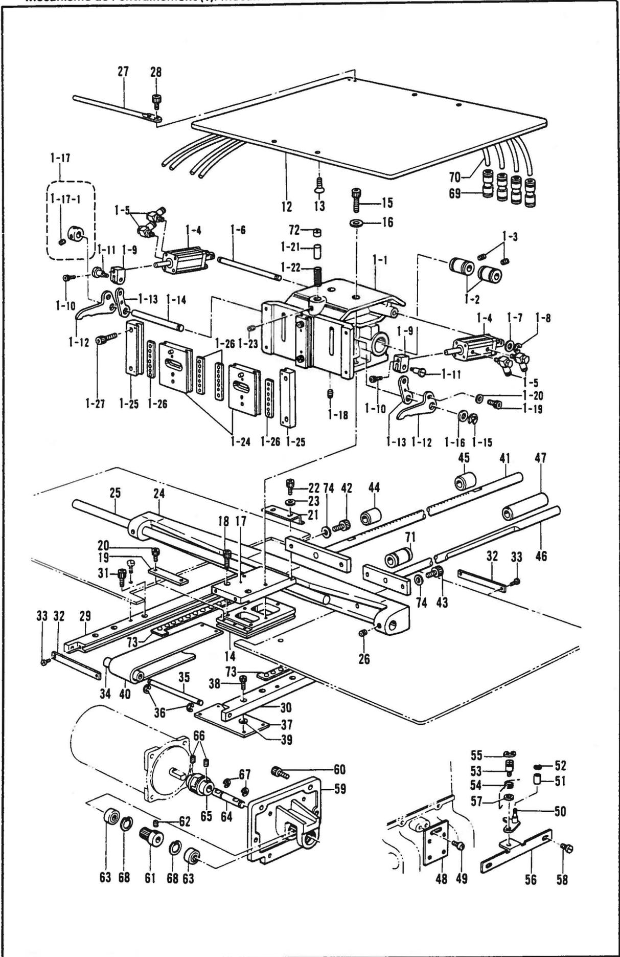
D1. 送り関係/Feed mechanism (1)/Transportvorrichtung (1)/
