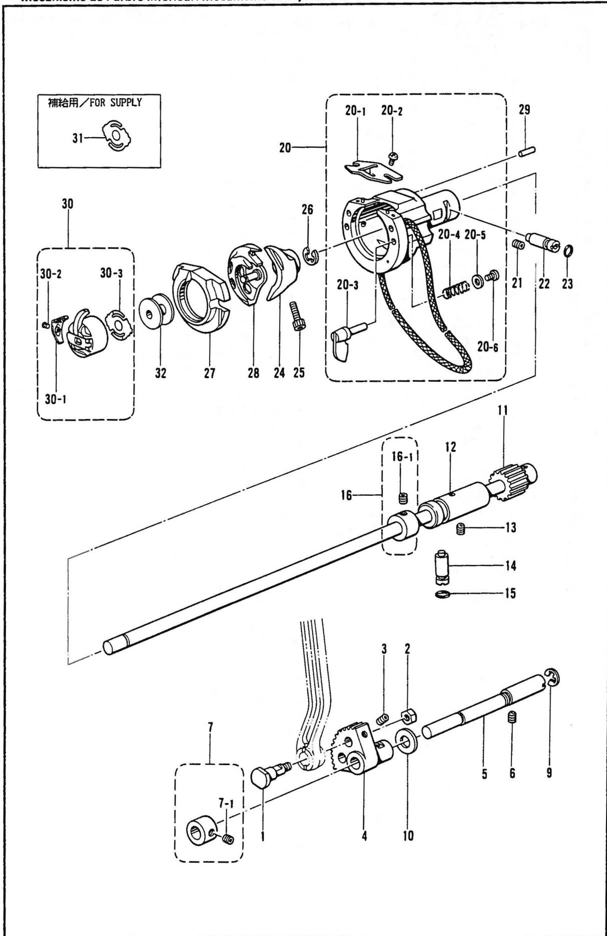
G. 下軸関係/Lower shaft mechanism/Untere Welle/
