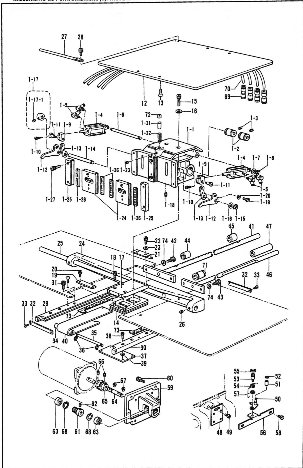
D1. 送り関係/Feed mechanism (1)/Transportvorrichtung (1)/
