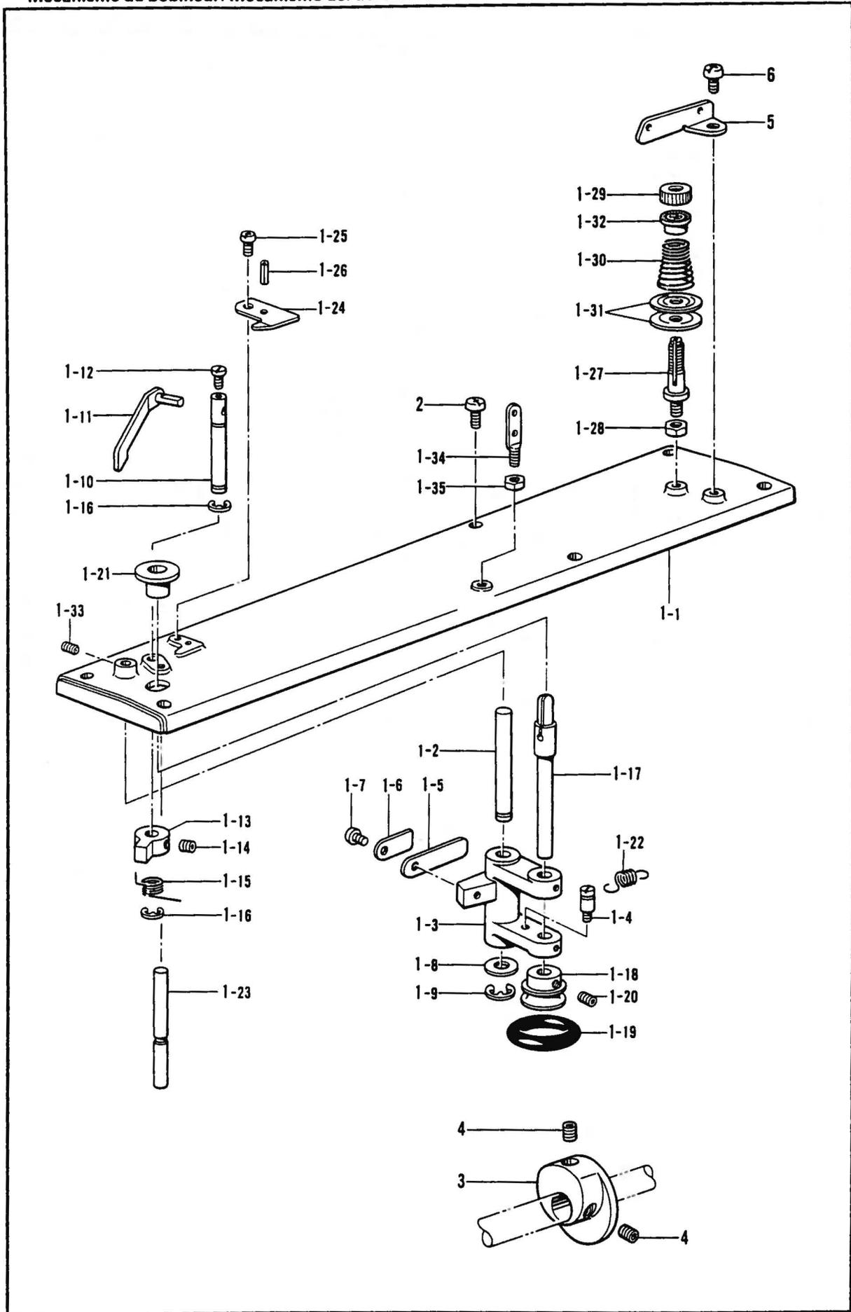
K. 糸巻キ関係 / Bobbin winder mechanism / Spuler /
